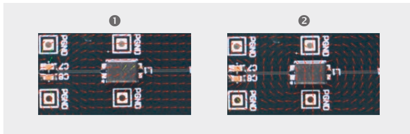
Figure 65 | Current vector at CMC without ESD protection at 1 ns ① and 15 ns ②. ESD is injected at the lower trace from the left side.
