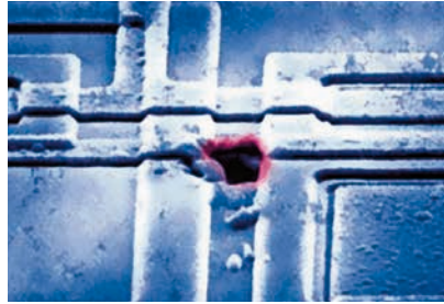
Figure 45 | Example of ESD damage
