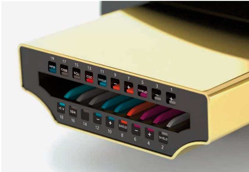
Figure 88 | Pinout and front view of HDMI connector
