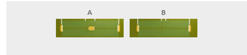
Figure 39 | Common routings for external ESD protection devices in leadless 3-pin package DFN1110D-3
